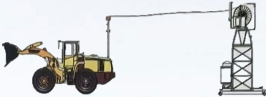
Electric suspended cable transmission system
