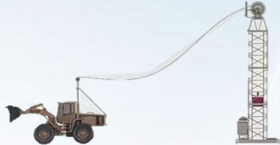
Heavy hammer cable drum transmission system
