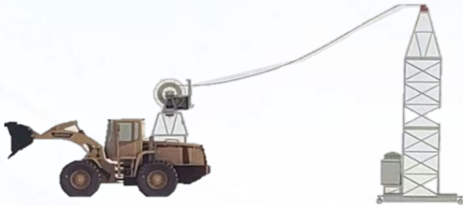
Vehicle mounted electric cable drum transmission system
